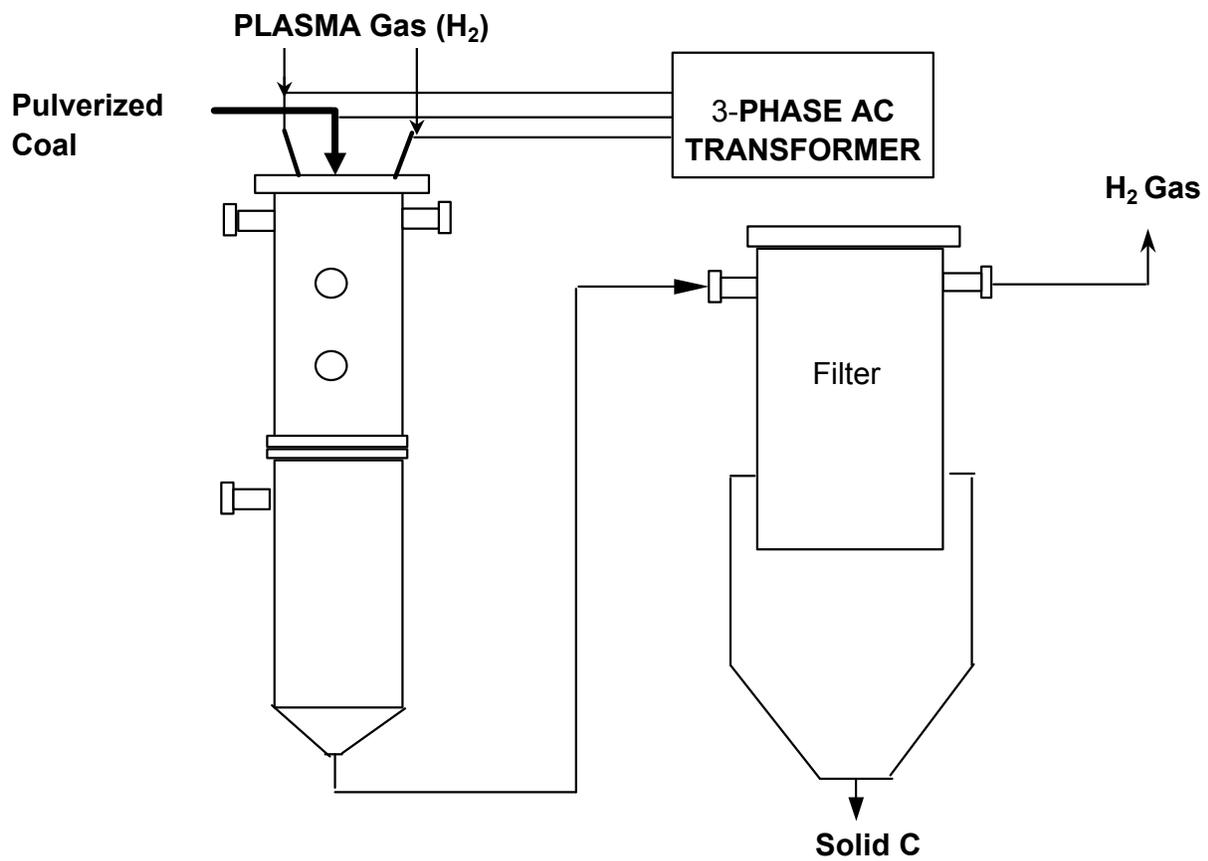
**Figure 2. THE HYDROGEN PLASMA BLACK REACTOR**
