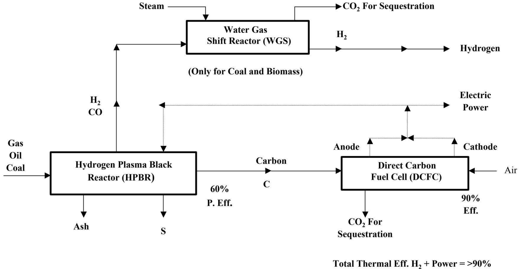
**Figure 5. IPFC Plant - Integrated Plasma Fuel Cell Combined Cycle
