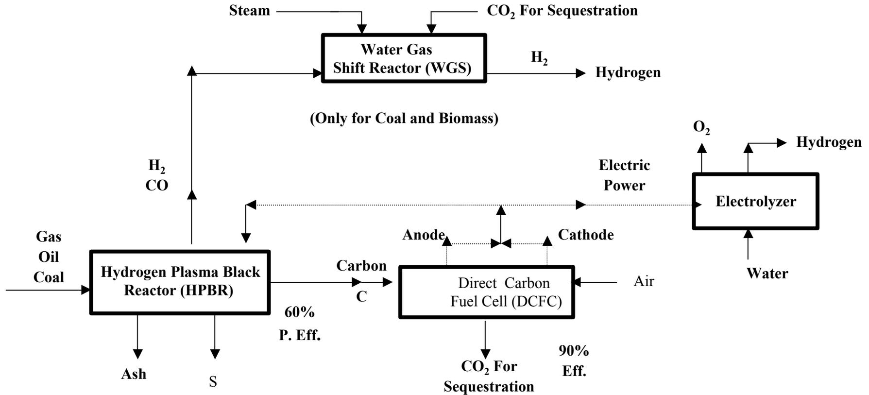
**Figure 6. IPFC Plant - Integrated Plasma Full Cell Combined Cycle for Hydrogen Production Only**
